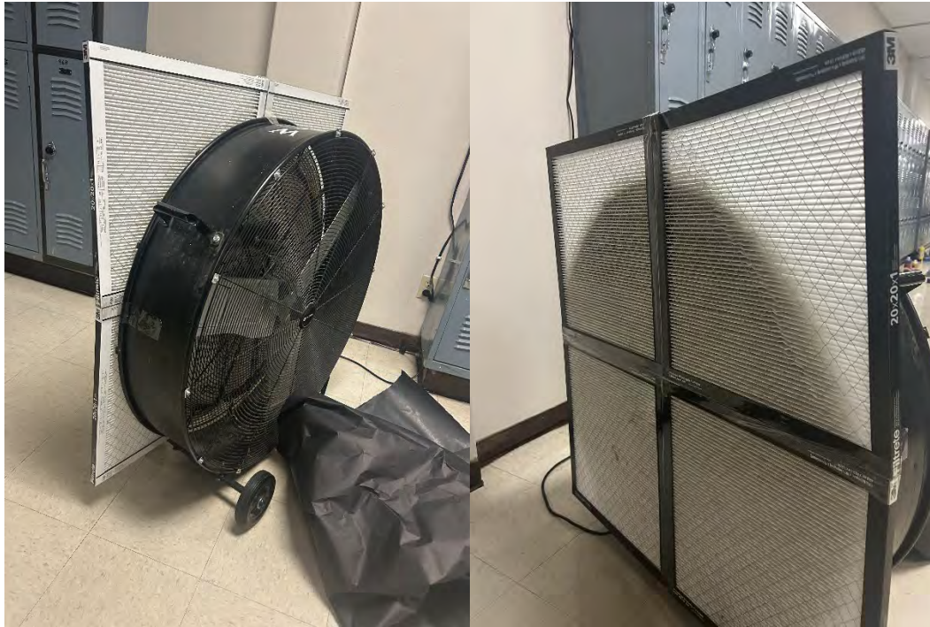
The photo above is an example of a Box Fan kit with MERV 13 filters after 24 hours of use.
